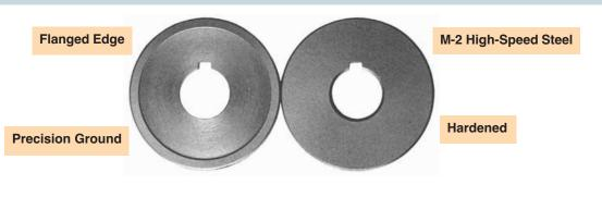
All saws, but especially those which are relatively thin, should be supported with as large as possible diameter flange support washers. These side support washers distribute the clamping force evenly, provide additional stability, and lessen the chance for deflection in thinner blades.
